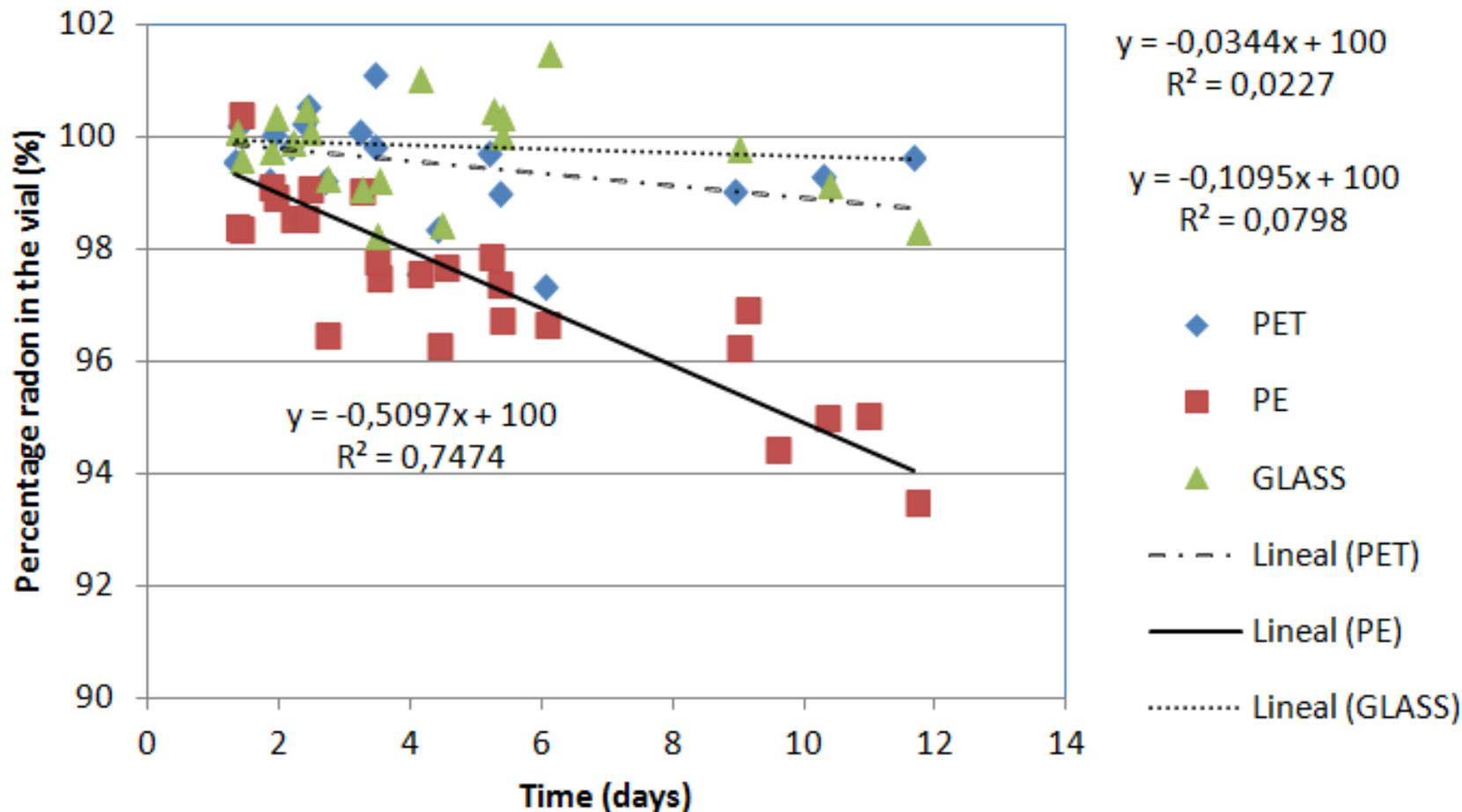
**$^{222}\text{Rn}$  determination for vials have been corrected for decay.**
