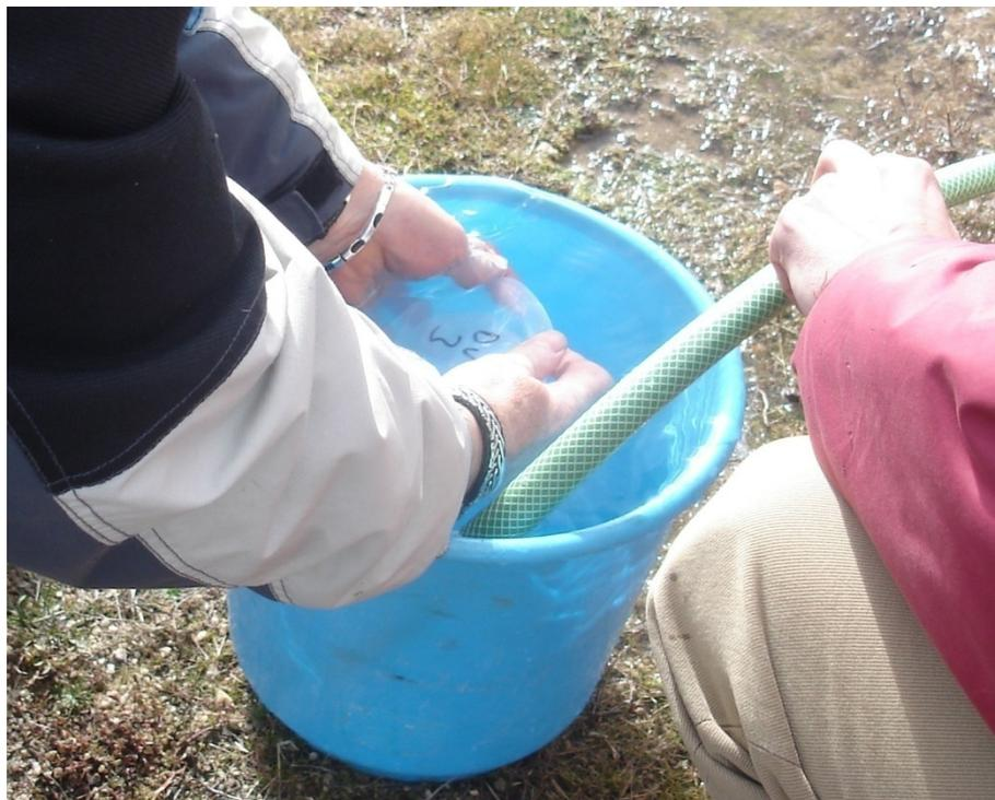
Samples were collected from the bottom of a container with two types of Marinelli beakers: 1.75 litres and 0.25 litres.
