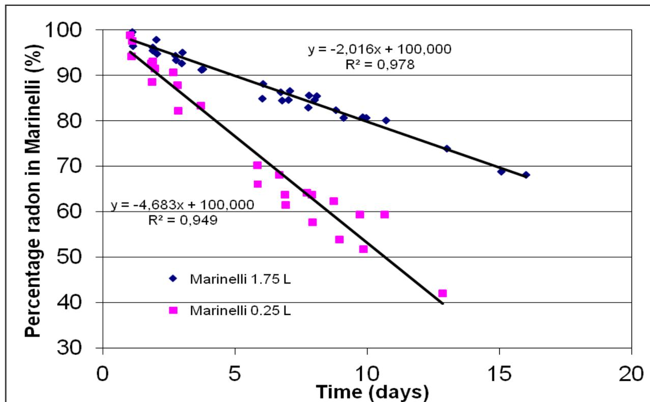
**$^{222}\text{Rn}$  determination for both Marinellis have been corrected for decay.**
