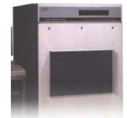
Counting was carried out using the liquid scintillation system Quantulus 1220™ from PerkinElmer. It is provided with a pulse-shape analyser (PSA) which separates pulsed caused by alpha or beta decays into different spectra, respectively.
