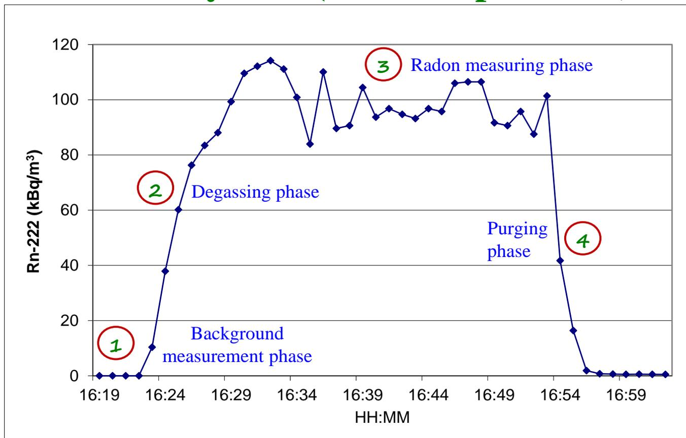
After less 10 minutes, equilibrium concentration is reached, then at least 10 more minutes the air circulate in the measuring system. After this time the pump is stopped and the system purged.
