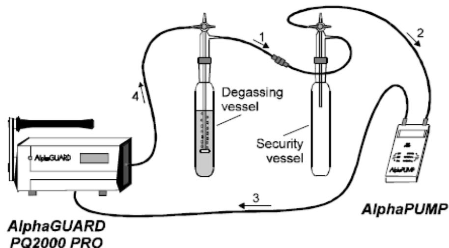
$$C_{water} = C_{air} \left( \frac{V_{air}}{V_{water}} + K_{water/air} \right) - C_b [Bq/l]$$
