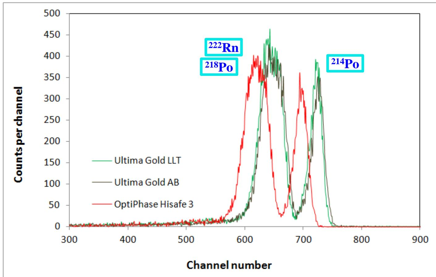
Any cocktail may be used for  $^{222}\text{Rn}$  measurements, although UG LLT and UG AB are more quench resistant than OptiPhase Hifase 3.
