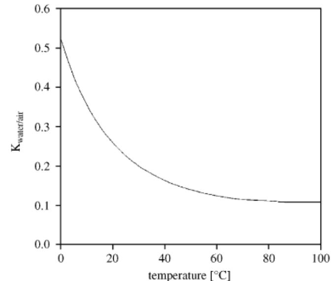
Dependency of the partitioning coefficient  $K_{water/air}$  on temperature (Clever, 1979)
