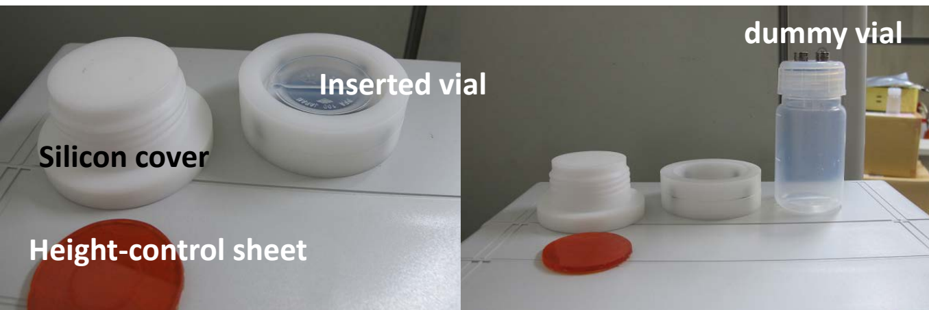
Top of the apparatus: the Teflon vial insert port
