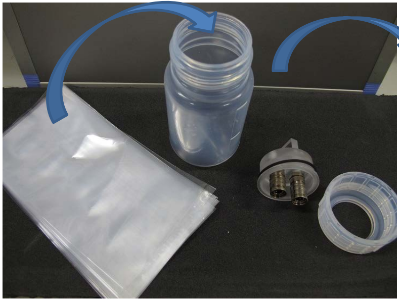
Polyethylene bags (75 mm × 150 mm × 0.3 mm), a Teflon vial with a special cap and plastic scintillator pellets
