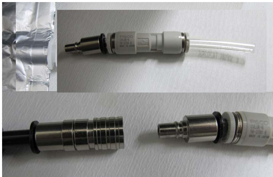
Top of the apparatus: the Teflon vial insert port
