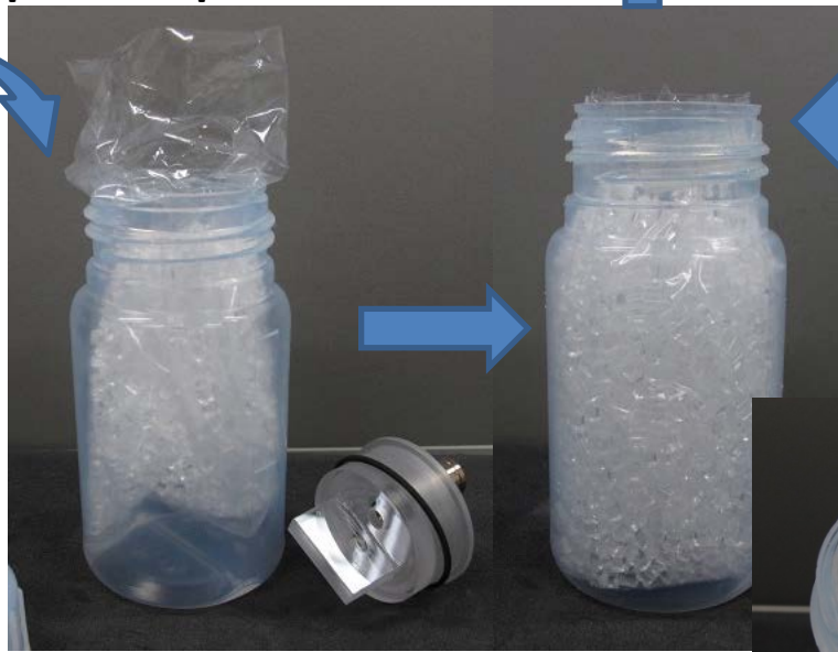
Polyethylene bags (75 mm × 150 mm × 0.3 mm), a Teflon vial with a special cap and plastic scintillator pellets
