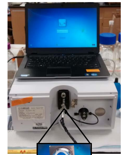
Flow scintillation analyzer (Online detection)
