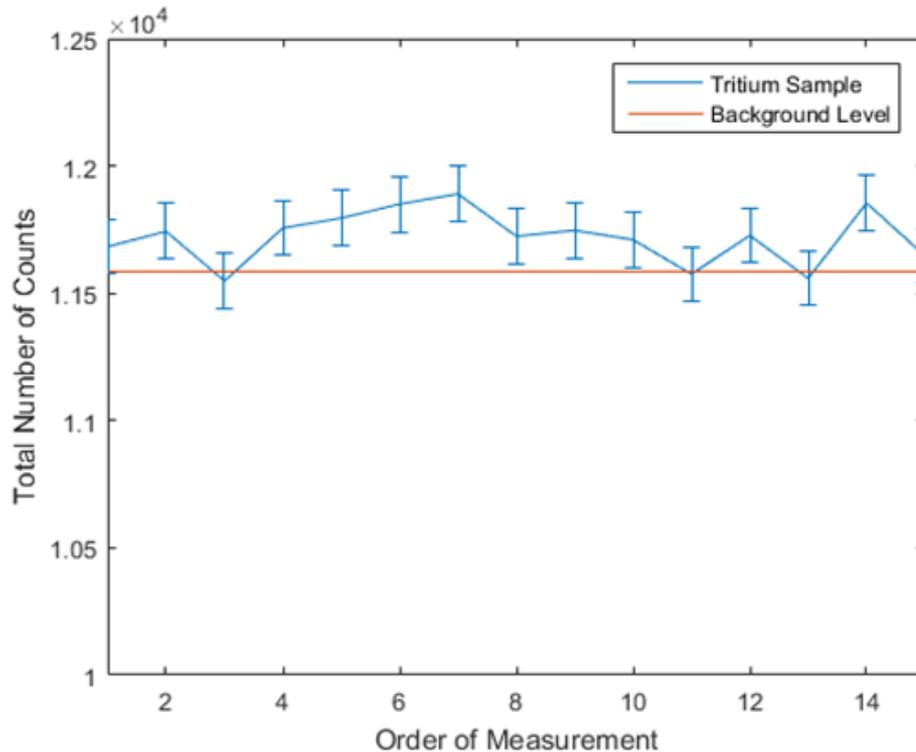
Fig. 9. Continuous measurement result for tritium gas sample.
