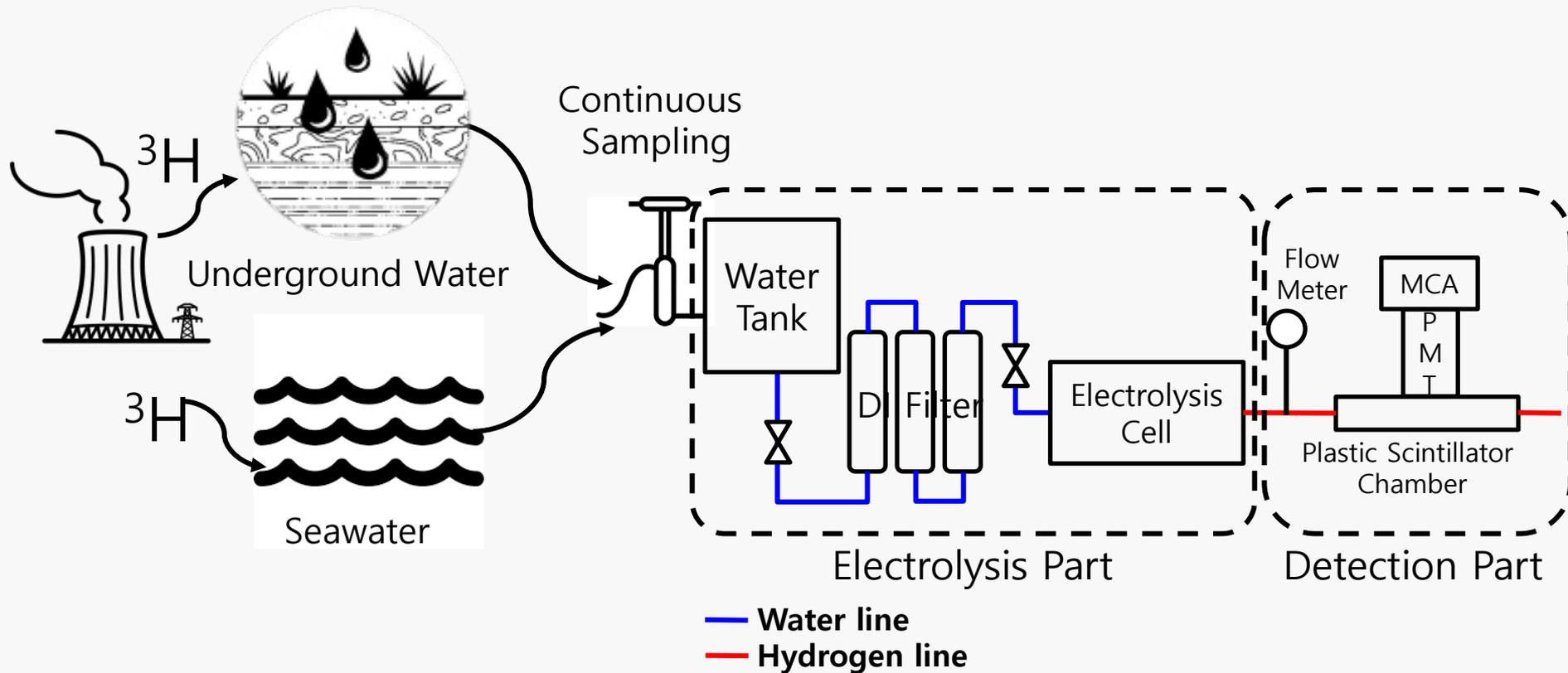
Fig. 3. Conceptual diagram of system for tritium continuous monitoring system using electrolysis and plastic scintillator detector.
