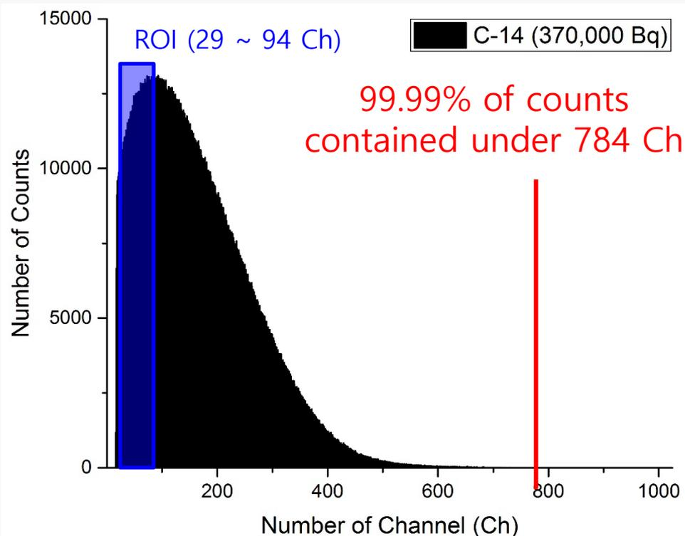
Fig. 8. Energy calibration using  $^{14}\text{C}$  source and range of interest (ROI) setup based on the tritium energy spectrum.
