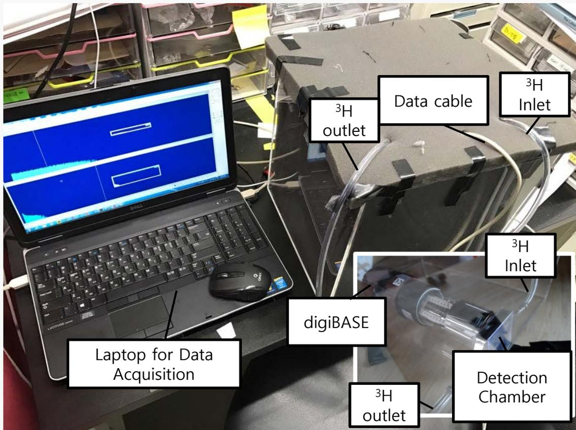
Fig. 4. Picture of the detector part
