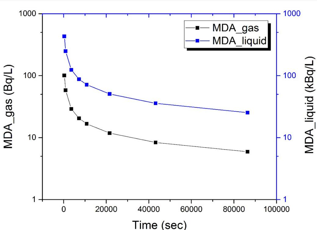
Fig. 10. Minimum detectable activity estimation curve for gaseous and liquid sample.
