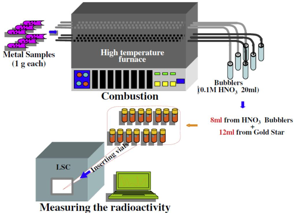
Fig. 2. A system for  $^3\text{H}$  trapping and measurement [1].
