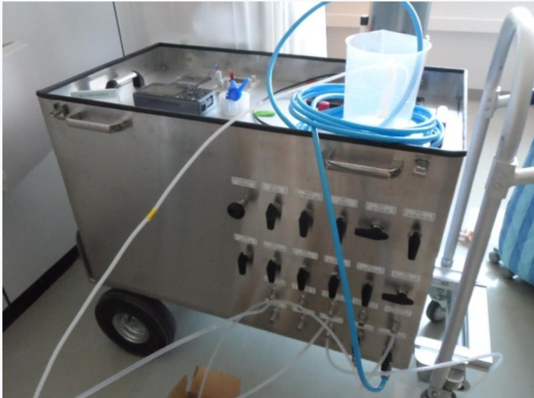
Fig. 5. Picture of the electrolyzer and continuous sampler system
