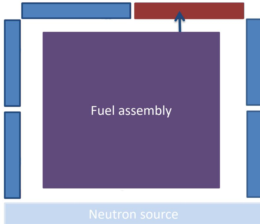
Detected coincident neutrons  $\rightarrow$  Fission events  $\rightarrow$  Fissile material
